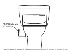
\*The 3-prong cord on the Washlet is on the right side and is 4' long. The GFCI outlet needs to have 120V, 10amps.
