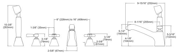
IMPORTANT NOTE: This valve/trim can only be installed in a built-up deck. It cannot be installed on pre-finished deck or on tub rim.
