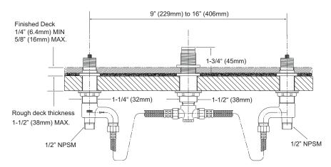
IMPORTANT NOTE: This valve/trim can only be installed in a built-up deck. It cannot be installed on pre-finished deck or on tub rim.
