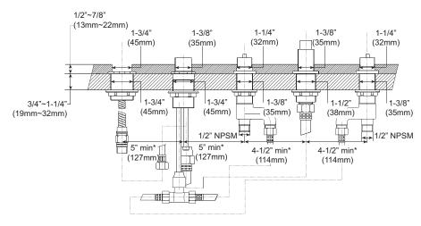
IMPORTANT NOTE: This valve/trim can only be installed in a built-up deck. It cannot be installed on pre-finished deck or on tub rim.
